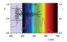
Perylene and benzoperylene carboxylic imides were arranged to form a bichromophoric dye with orthogonal electronic transition moments. However, quantitative Förster-type energy transfer (FRET) proceeds in spite of this orthogonality.
